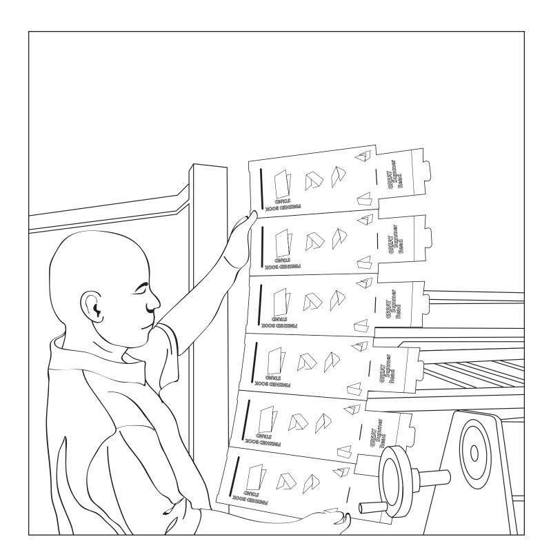
Boxes and point of purchase displays are manufactured by cutting, folding, printing and gluing corrugated sheets using a flexo-folder gluer or diecutter. Once the boxes or displays are manufactured, they are shipped to the customer. Based in Central Florida, Central Florida Box Corporation is a leading provider of packaging and display products.
